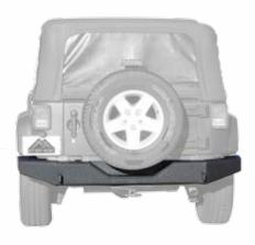
RT Off-Road's Rear Bumper is a heavy duty steel constructed upgrade over the factory bumper. The 3/16" plate steel construction is protected with a durable textured black powder coat finish. This rear bumper includes mounting points for D-rings and a large recess for oversized tire clearance. Includes all hardware needed for installation, installs into factory locations, and does not require any drilling or modification.
